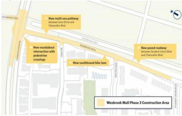
A new roundabout replacing the existing intersection of Wesbrook Mall and Chancellor Boulevard; pedestrian crossings across all sides of the intersection; a continuous bike lane in the southbound direction and improved conditions for cyclists in the northbound direction.
